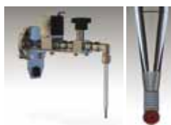
Enzyme Kinetics Probe - Real time mass spectrometry for enzyme kinetics studies
