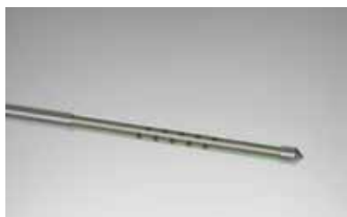
DEMS - Differential electrochemistry inlet for mass spectrometry
