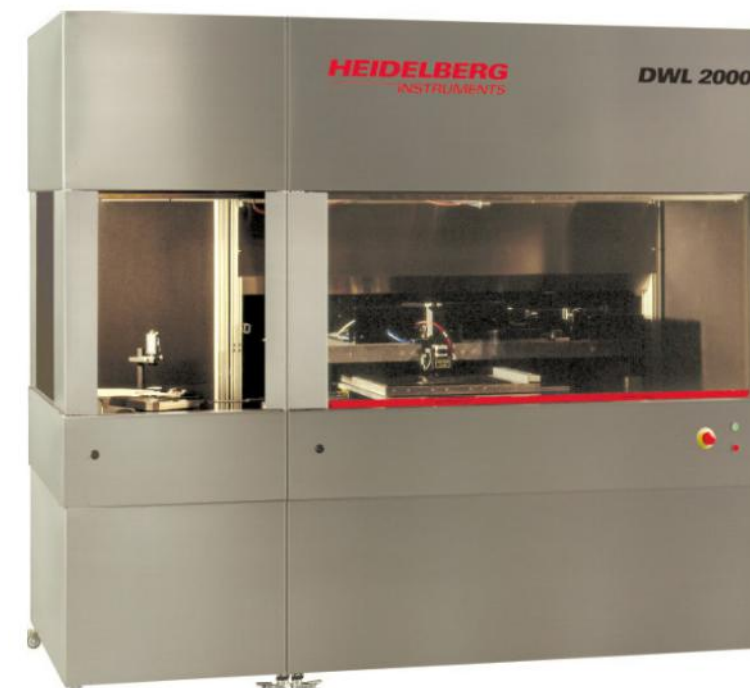
The new Heidelberg Instruments DWL 2000 laser pattern generator can expose substrates up to 200 mm x 200 mm for use in the stepper or for contact lithography, and has the ability to write patterns directly on substrates. It can expose photomasks with feature resolution down to 700 nm at speeds up to 110 mm 2 per minute.
