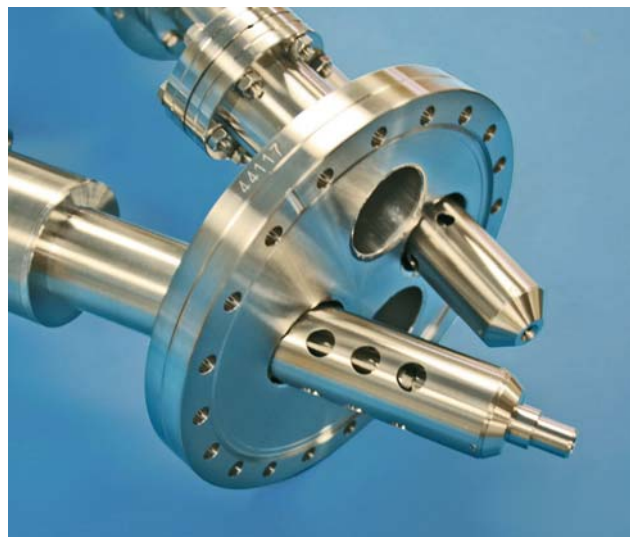
A complete SIMS/SNMS facility mounted on a single conflat flange
