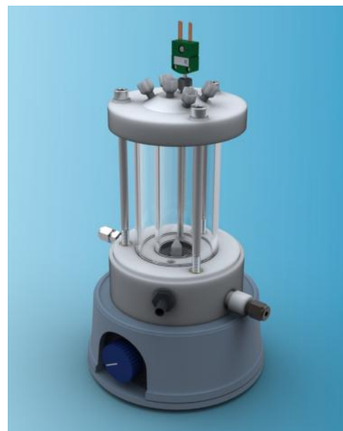
Cuvette style cell with water cooling jacket
