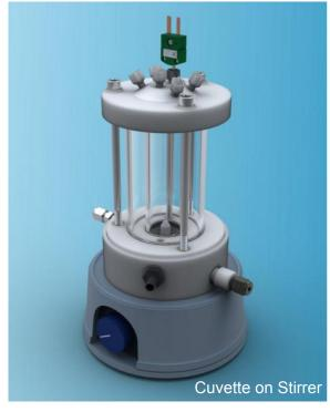
included to enable measurement with illumination excluded. Two membrane holders are also supplied to provide a 4-fold difference in membrane surface area, the larger area being preferred for enhanced transmission of organic vapors and the smaller for dissolved gas measurement. Connectors are included for water connectivity and thermocouple insertion.
