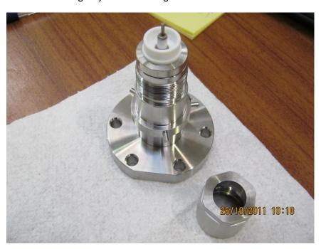
8 Next remove the ceramic spacer/insulator.
