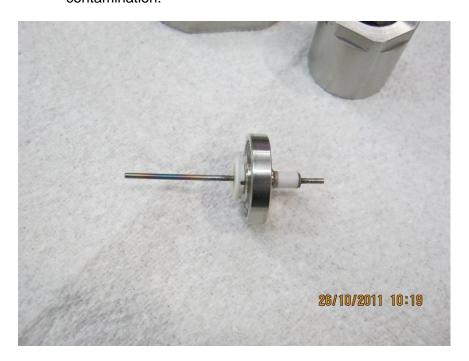
11 Next remove the Copper gasket for replacement when re-assembling.
