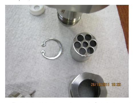
13 The body should then be turned over so the Cathode plate can be removed from the body, which should fall out.
