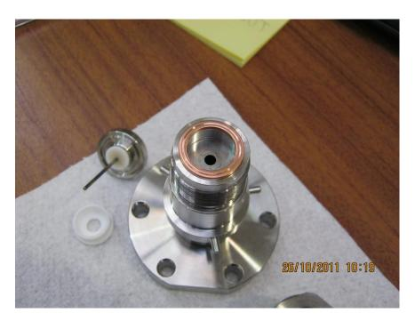
10 The Anode can be cleaned by using a fine abrasive paper (600 Grade) on the pin section and a fiberglass pen on the ceramic section, depending on the contamination.
